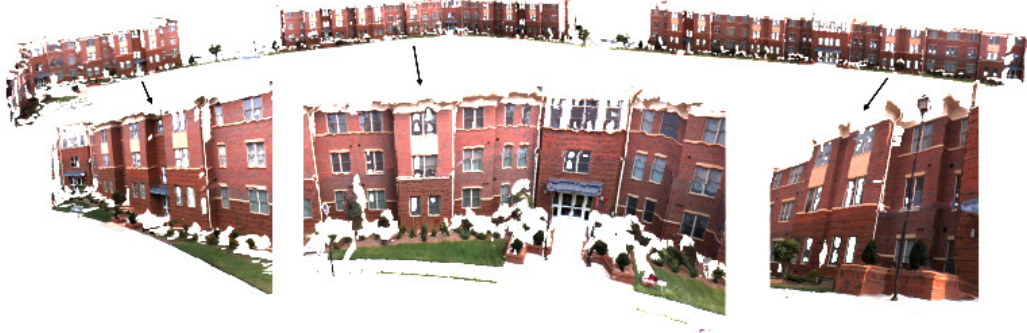
Figure 1.1: 3D model of the facades in a street side, obtained on-line from a moving vehicle with the system described at [Akbarzadeh et al., 2006]. The reconstruction application runs on an on-board computer, equipped with a powerful Graphical Processing Units (GPU's), and obtains a simplified 3D model of the street, consisting on planar surfaces detected at the building facades.
