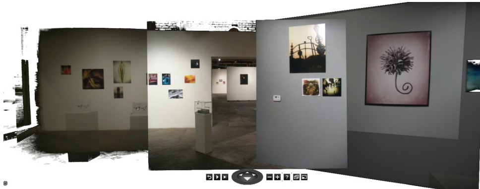
Figure 1.4: Navigable image mosaic, generated with Photosynth [Labs, 2012] from pictures captured inside an art gallery. Photosynth is an on-line application based on the Phototourism project for SfM reconstruction [Snavely, Seitz and Szeliski, 2006]. The application renders on an image mosaic the approximate visual appearance of the scene, as seen from a given view point. The user can change this view point using the interface to navigate through the scene in a simulated virtual presence.
