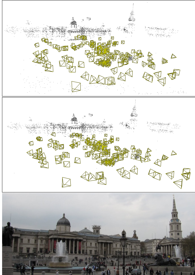
Figure 5.17: Camera poses and detail of the sparse scene structure obtained from the dataset trafalgar-161 , using the following methods: Top: correction of the camera poses contained in the dataset with GEA, and re-estimation of the structure with the linear triangulation. Middle: incremental motion estimation and the linear structure triangulation from the pairwise matching information contained in the dataset. Bottom: picture from the original scene (Author: https://ssl.panoramio.com/user/3029536 ).
