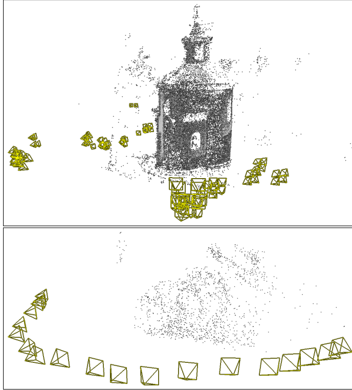
Figure 5.18: Sparse reconstructions obtained for the video sequences stmartin ( top ) and medusa ( bottom ) using the structureless incremental motion estimation procedure, and the linear structure triangulation.
