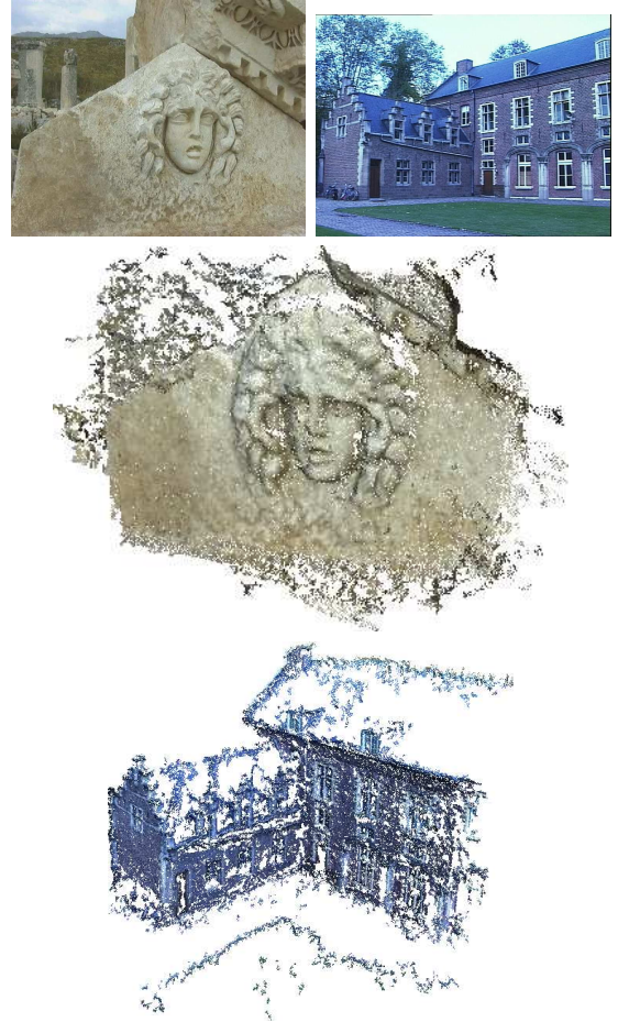
Fig. 6. Top row: sample images from the data-sets medusa and leuven castle (top row). Middle and bottom: dense reconstructions obtained for these data-sets using the PMVS2 software, and the camera poses provided by the incremental motion estimation procedure.
