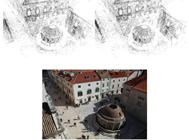
Figure 1. Visual comparison of the reconstruction obtained with sSBA and GEA. SfM reconstruction of the fountain optimized with sSBA, and optimized with GEA using linear estimation of the 3D points (top row left and right image respectively). Top view of the Onofrio fountain at Dubrovnik (bottom image).
